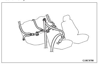
The UNIBELT at the rear seat positions, and at the front passenger seat, can be converted from normal Emergency Locking retractor (ELR) mode, to Automatic Locking Retractor (ALR) mode. It must be converted to the ALR mode when installing a child restraint system.
